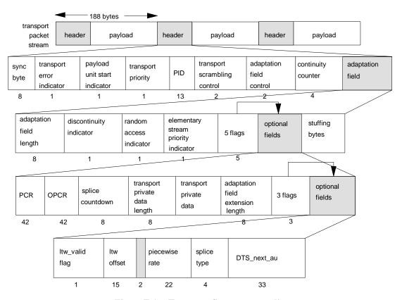
Figure F-1 -- Transport Stream syntax diagram
