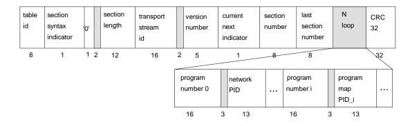
Figure F-3 -- Program association section diagram
