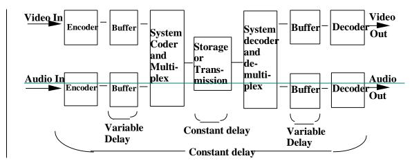
Figure D-1 -- Constant delay model
