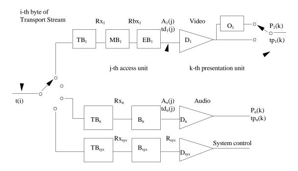
Figure 2-6 -- Transport Stream system target decoder notation
