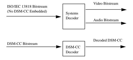
Figure A-2 -- DSM CC bitstream decoded as a standalone bitstream
