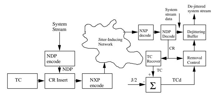
Figure K-2 -- Jitter smoothing using network-layer timestamps
