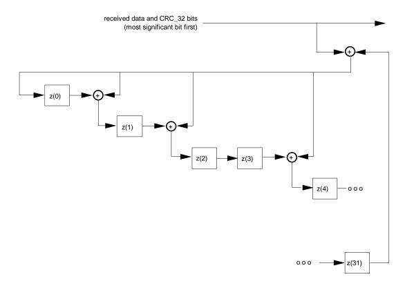
Figure B-1 -- 32 bit CRC decoder model
