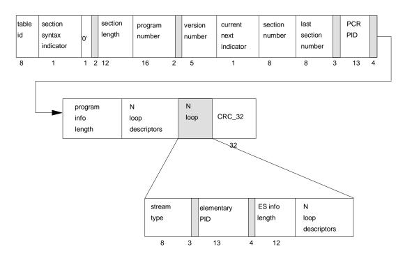
Figure F-5 -- TS program map section diagram
