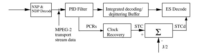
Figure K-3 -- Integrated dejittering and MPEG-2 decoding
