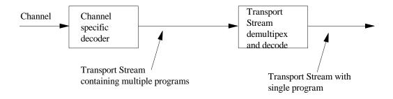
Figure 0-3 -- Prototypical transport multiplexing example
