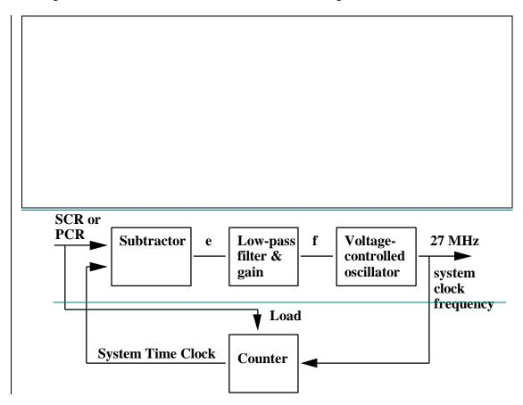
Figure D-2 -- STC recovery using PLL
