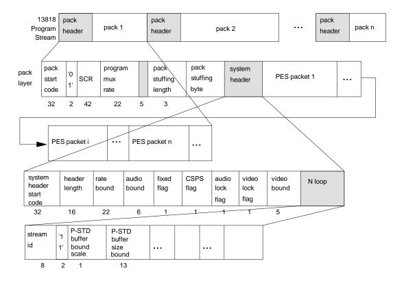
Figure F-7 -- Program Stream diagram
