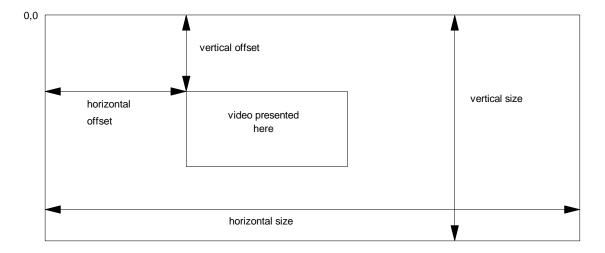
Figure 2-8 -- Target background grid descriptor display area
