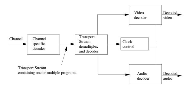
Figure 0-2 -- Prototypical transport demultiplexing and decoding example
