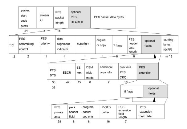
Figure F-2 -- PES packet syntax diagram
