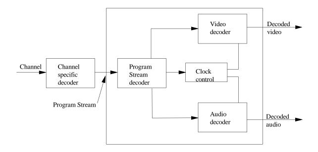
Figure 0-5 -- Prototypical decoder for Program Streams
